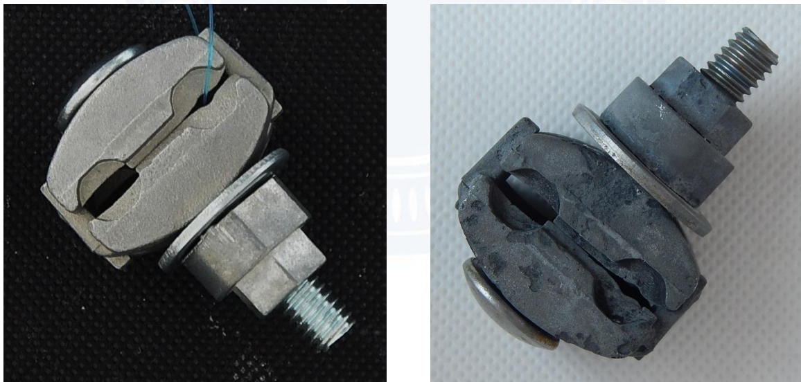
Figure 13. Visual appearance of sample 21MA0034-10 . Initial (left) and final (right) appearance.
