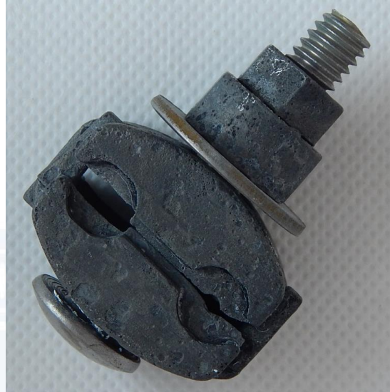
Figure 6. Visual appearance of sample 21MA0034-3 . Initial (left) and final (right) appearance.
