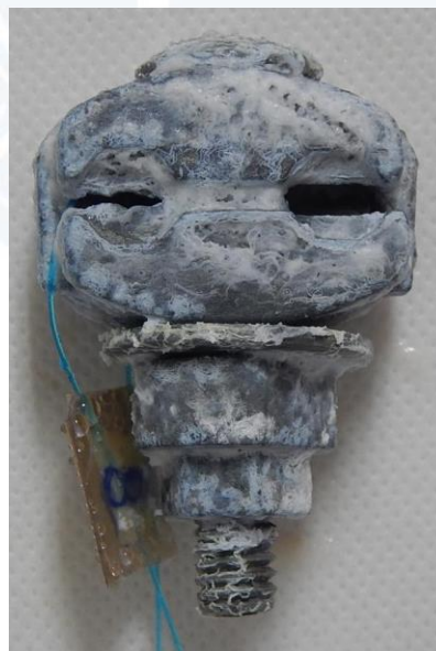
Figure 3. Visual appearance of sample 21MA0034-9 at 150 hours of test
