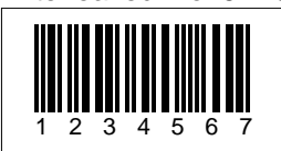
Interleaved 2 of 5 + CHECKSUM
